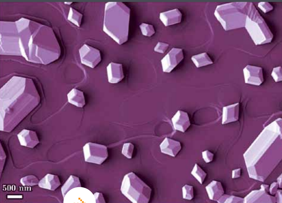
W particles (false color) on a sapphire substrate in the presence of anorthite ( \text{Al}_2\text{O}_3 - \text{CaO} - 2\text{SiO}_2 ), acquired using the LEO by Amir Avishai (Prof. Wayne D. Kaplan).
