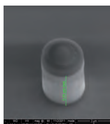
Figure 2 (Left). Scanning electron microscope image of a single photonic pillar containing single QD. (Right) Polarization sensitive PL spectra from the micropillar under high excitation power. The blue (green) line presents H (V) linear polarization.
