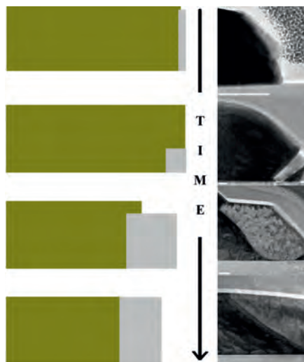
Figure 1. Qualitative comparison between kinetic model and experiment: the time-evolution of an Fe nucleus, which grows with time and undergoes a transition from inside to outside of the Au particle. The scale bars are 50 nm. The brighter phase in the TEM images represents Fe [3].
