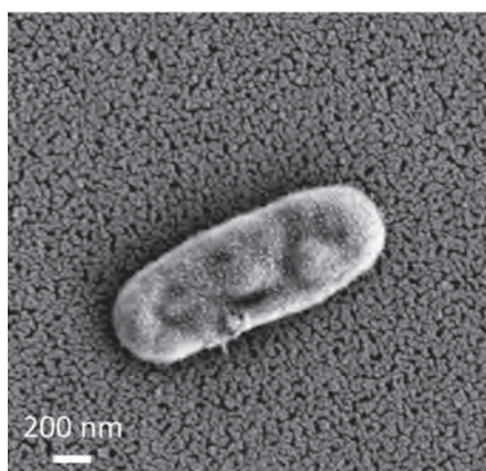
Figure 1. High-resolution scanning electron micrograph of an E. coli cell captured on the surface of a porous Si optical transducer.
